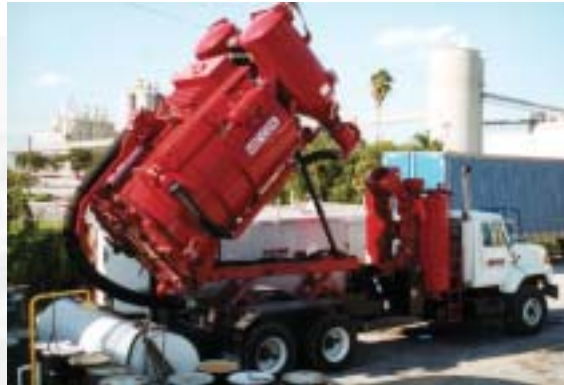
SWS recently acquired this new VAC-CON industrial loader unit specially equipped with a hydraulic, rear mounted, pendant control, high dumping system. This unique high dumping system allows liquids and solids within the tank to be dumped directly into 60" containers without having to pull onto ramps, berms, elevations, etc. This new unit is ideal for performing hydro and air systems excavation.
